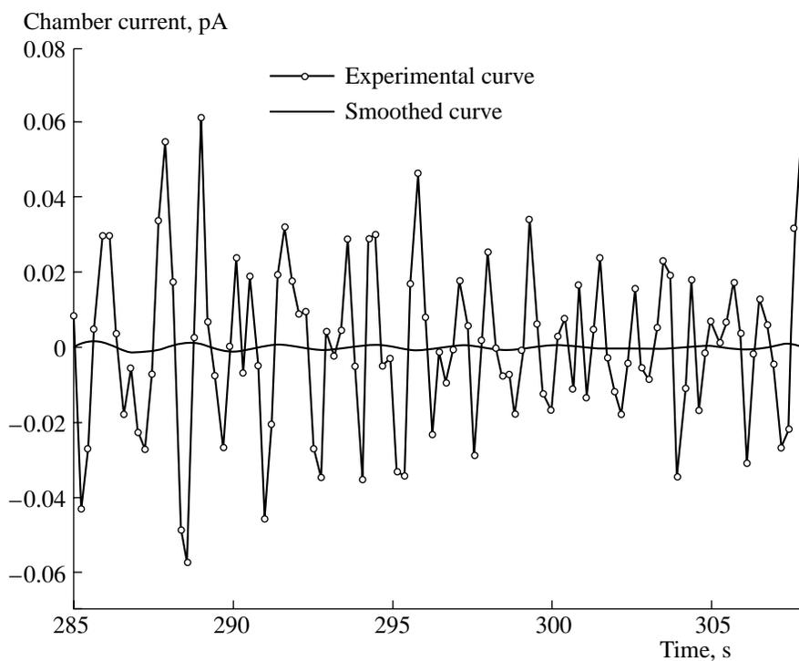
**Fig. 11.** Noise characteristics of measuring channel with an electrometric amplifier.
