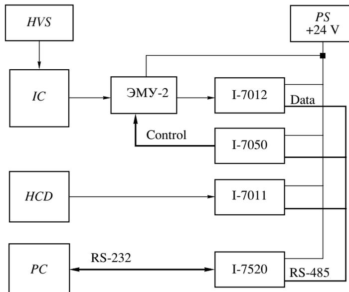
Fig. 10. Block diagram of molecular composition monitor: (PC) personal computer; (HVS) high-voltage supply; (IC) flow-type ionization chamber; (ЭМУ-2) electrometric amplifier with band switching; (PS) power source (+24 V); (HCD) heat-conductivity detector; (I-7011) analog-input module; (I-7520) RS-232/RS-485 interface converter.
