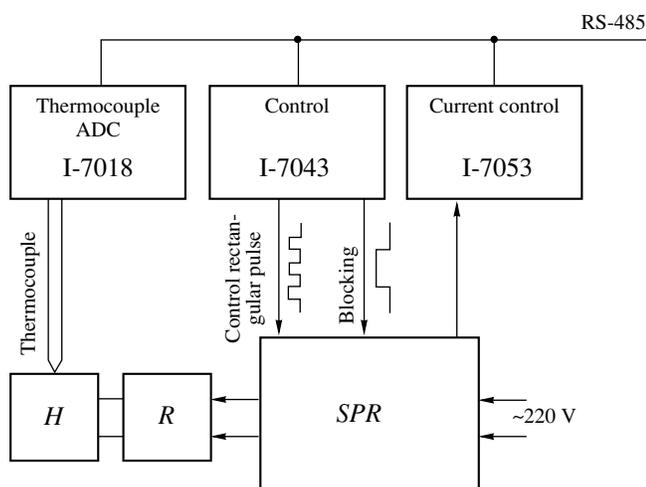
**Fig. 2.** Block diagram of the heating-control circuit: (*SPR*) semiconductor power regulator; (*R*) heater-blocking relay; (*H*) heater; (I-7018) multichannel analog-input module; (I-7043) multichannel digital-output module; and (I-7053) multichannel digital-input module.
