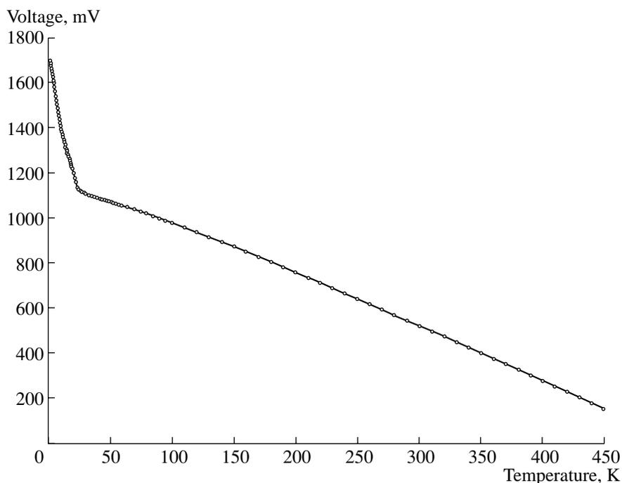
**Fig. 7.** Standard temperature characteristics of a thermodiode (a D 200 19 707 LEYBOLD silicon diode).
